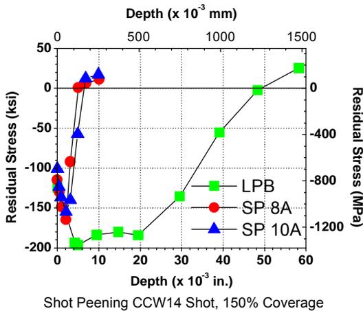
Figure 1 - Residual stress distribution for SP and LPB processed specimens showing 10X greater depth and 30% greater peak compression for LPB process compared to shot peening.
