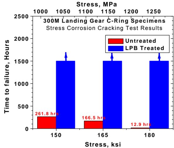
Figure 3 - SCC test results.
