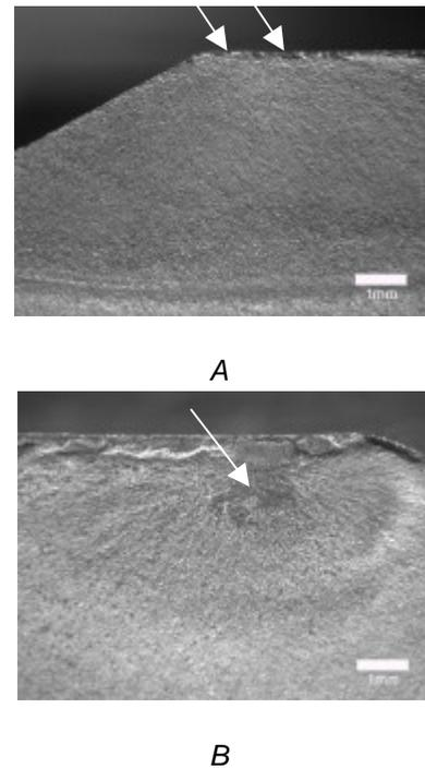
Figure 4 – (A) Fracture surface of shot peened specimen showing multiple surface initiations indicated by the arrows. (B) Fractograph showing subsurface initiation in LPB specimen.
