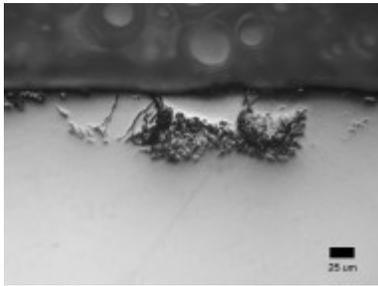
Figure 5 – Cross sectional view of a typical corrosion pit in a shot peened corrosion fatigue test specimen.
