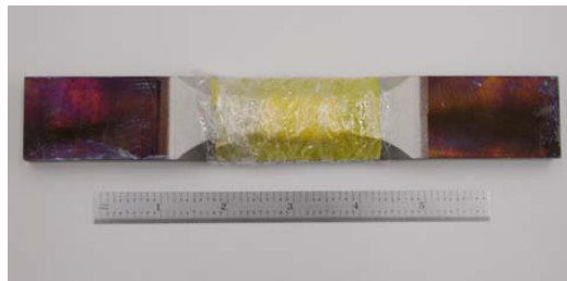
Figure 2 - A Type 1 HCF specimen with 3.5% salt solution soaked tissue wrapped around the gage section to produce an 'active corrosion' environment during fatigue testing.
