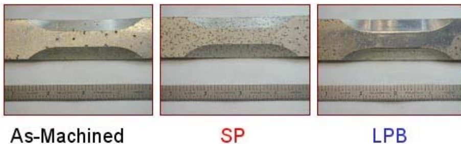
Figure 4 – AA7475-T7351 fatigue specimens after exposure. SP specimens exhibited greater corrosion damage than LPB and as machined specimens.
