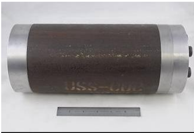
FIGURE 5: FULL SIZE COUPLING BLANK PLACED IN PRESSURIZED TEST APPARATUS.
