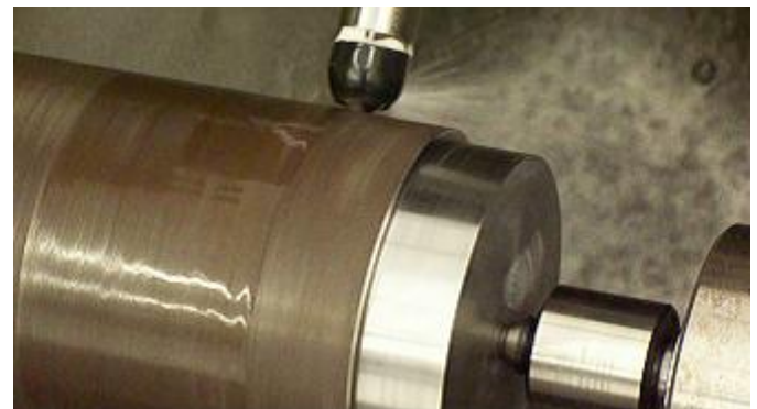
FIGURE 2: API-P110 COUPLING BEING LPB PROCESSED ON A CNC LATHE
