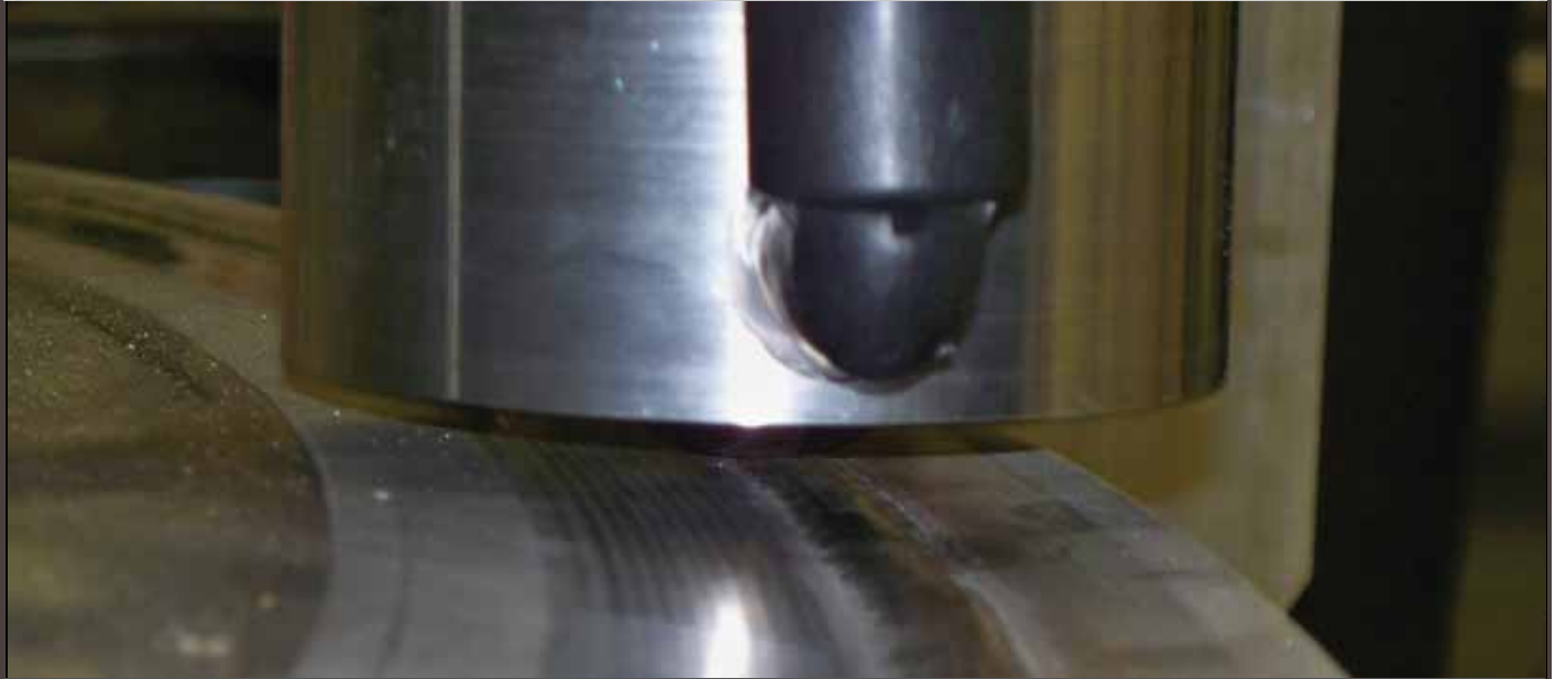
Lambda-designed tool impinging residual stresses in a radioactive waste container weld
