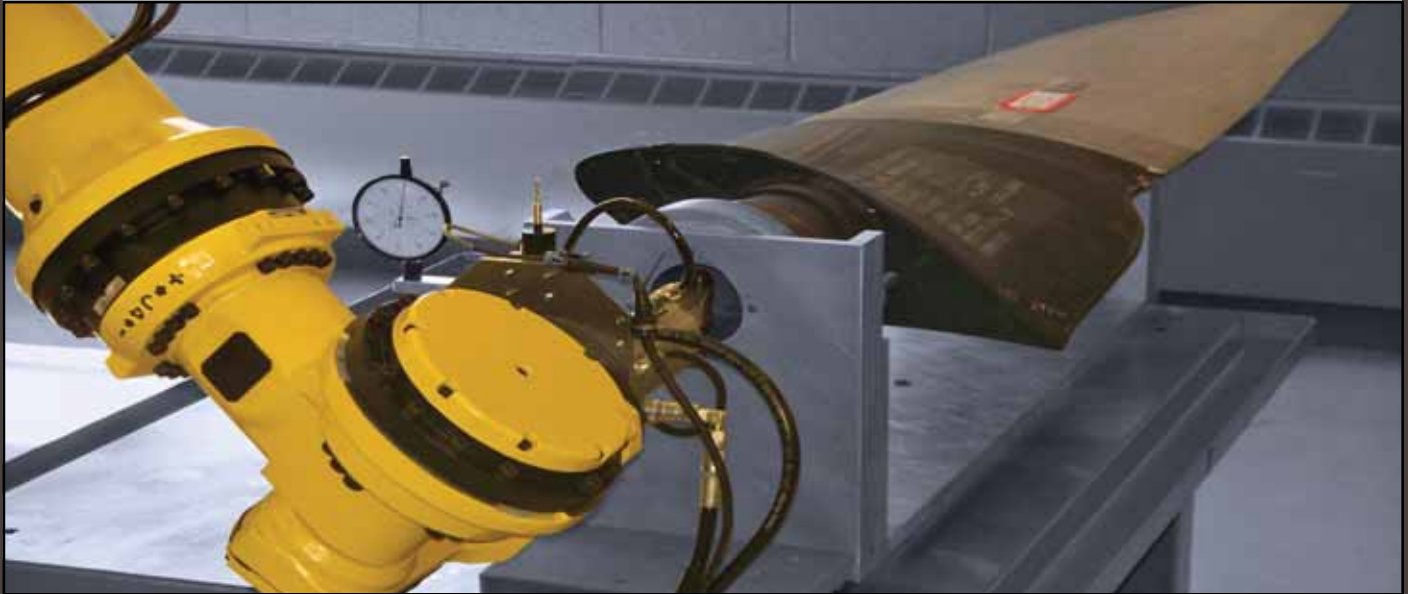
LPB processing of an aluminum alloy propeller blade
