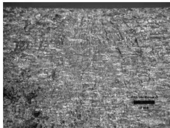
Figure 7: Fracture face showing typical surface failure for milled specimen.
