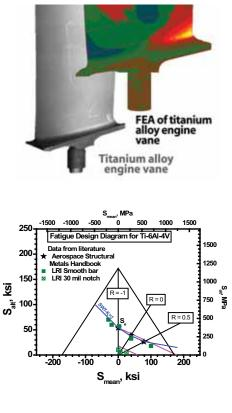
The Fatigue Design Diagram (FDD) provides a means of designing compressive residual stress distributions into metallic components necessary to achieve optimal fatigue performance and to mitigate typical damage conditions.
