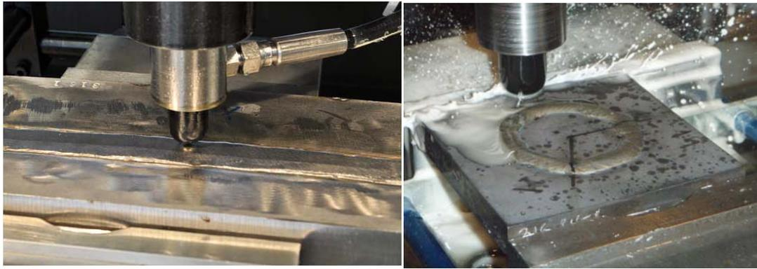
Figure 1: LPB Processing of specimens
