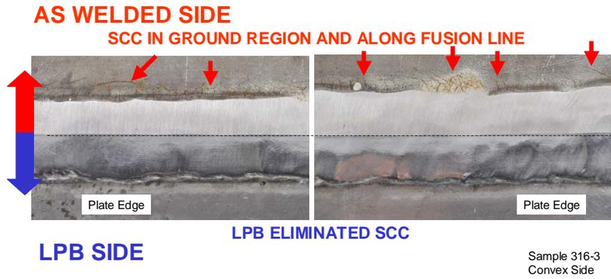
Figure 13: Close-up of Sample 316-3 fusion line on convex side following  $MgCl_2$  exposure revealing SCC along fusion line and in ground regions on untreated side and no SCC on LPB side.
