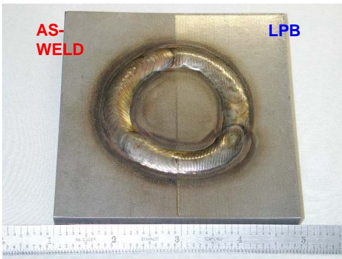
Figure 1 – 316L circular weld specimen
