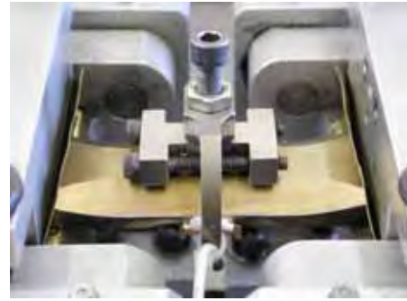
FIG. 13. Fretting fixture with instrumented loading ring and bridge device to hold two fretting cylindrical pins clamped on to the fatigue specimen surface under a controlled normal force.
