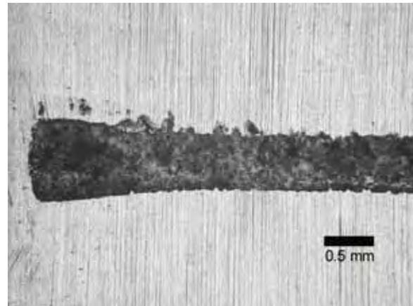
FIG. 16(b). Typical fretting scar on LPB surface. ( S_{max}=78 ksi and N_f=1,550,922 )
