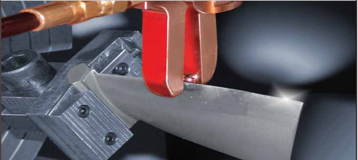
LPB processing of a stainless steel 1st stage compressor blade in the T56 turboprop engine
