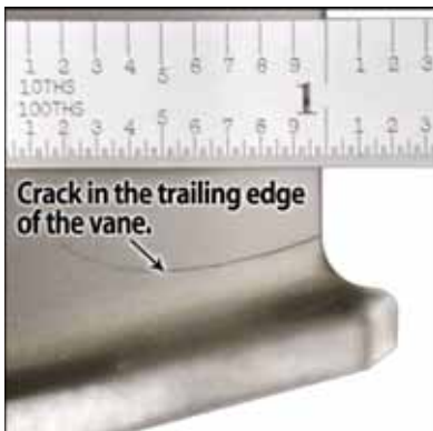
Vane axial stress due to combined bending and torsion in engine service.
