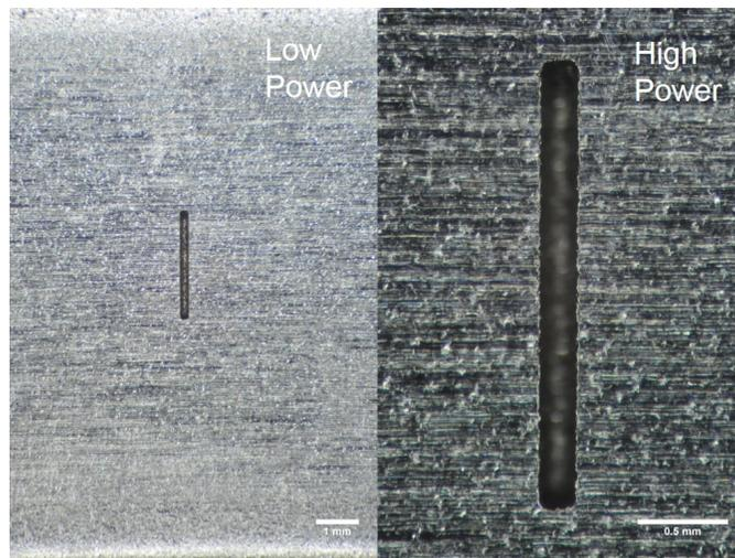
**Figure 2: Mid-Gage EDM Notch in HCF Ground Specimen**
