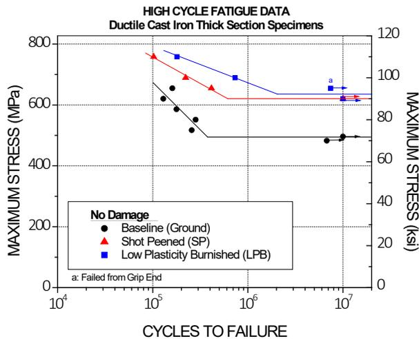
**Figure 5: High Cycle Fatigue Results of Ductile Cast Iron Specimens With No Damage**
