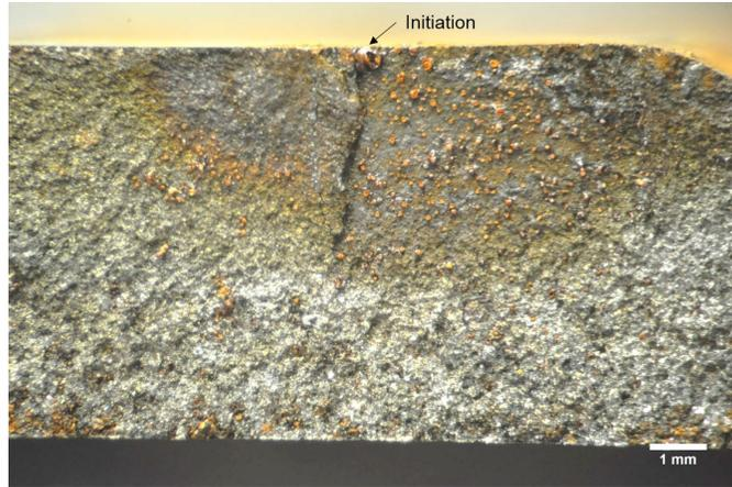
**Figure 15: Fracture Face of an LPB Specimen With a 0.010 in. Deep Notch Ran in CF**
