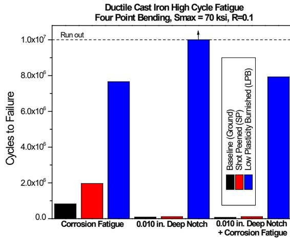
Figure 10: High Cycle Fatigue Results at Smax= 70 ksi
