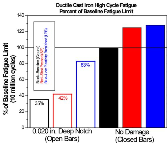
Figure 7: High Cycle Fatigue Results of Ductile Cast Iron Specimens Plotted as a Percentage of the Baseline Fatigue Limit
