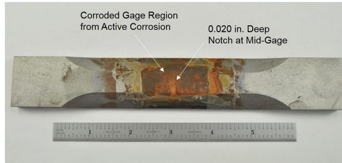
**Figure 3: Actively Corroded LPB Processed HCF Specimen After Testing to Run-Out**
