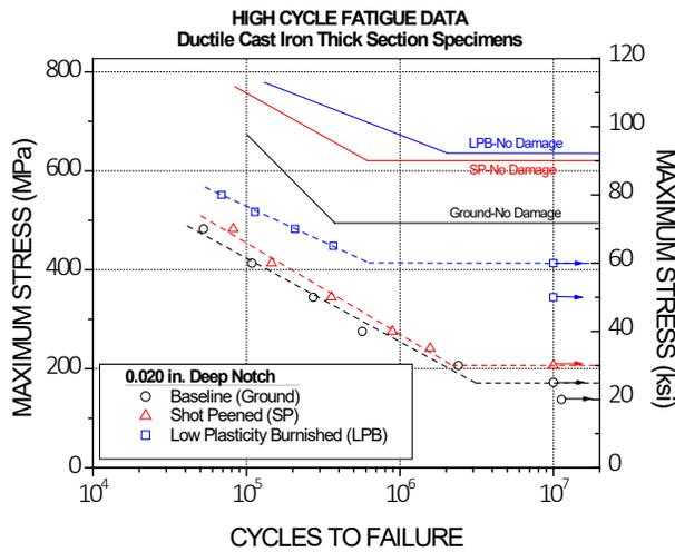
Figure 6: High Cycle Fatigue Results of Ductile Cast Iron Specimens with 0.020 in. Deep Notches
