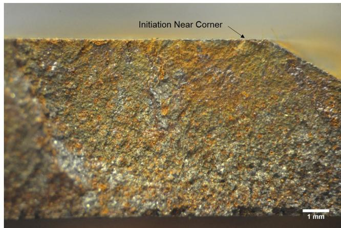
**Figure 13: Fracture Face of a LPB Specimen Ran in CF**
