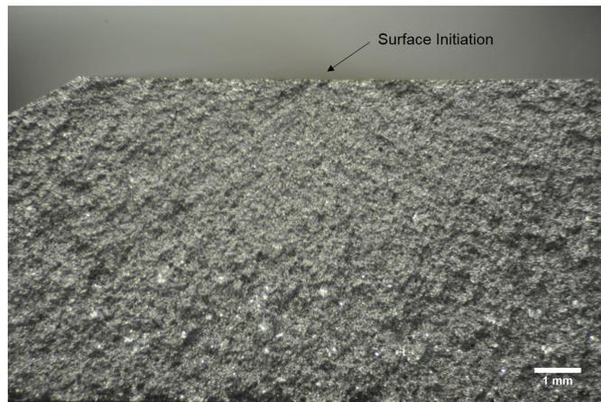
Figure 11: Fracture Face of a Baseline (Ground) Specimen
