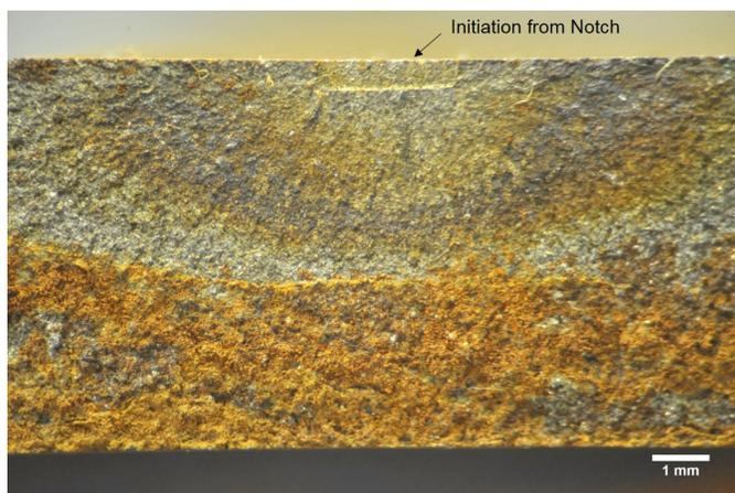
**Figure 14: Fracture Face of a Shot Peened Specimen With a 0.020 in. Deep Notch Ran in CF**
