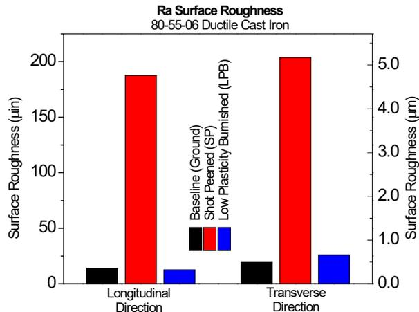
**Figure 17: Surface Roughness of Ground, Shot Peened, and LPB Processed Surfaces**
