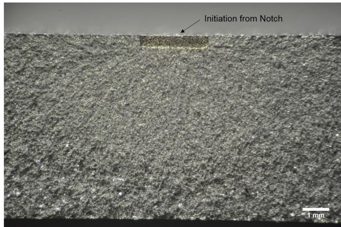
**Figure 12: Fracture Face of a Shot Peened Specimen With a 0.020 in. Deep Notch**
