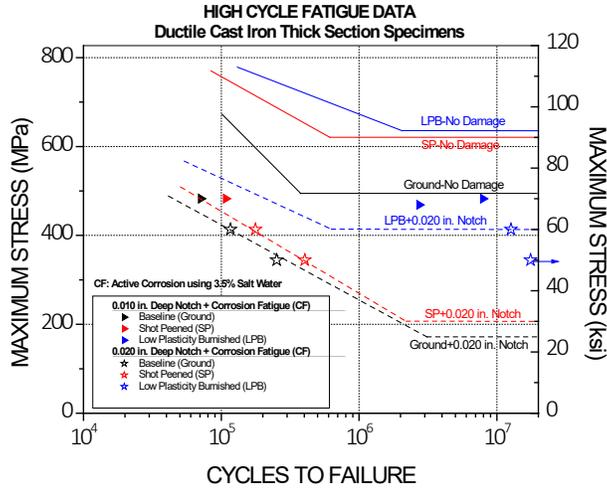
Figure 8: High Cycle Fatigue Results of Ductile Cast Iron Specimens With 0.010 in. and 0.020 in. Deep Notches and Corrosion Fatigue (CF)
