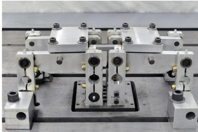
**Figure 4: High Cycle Fatigue Four Point Bending Test Fixture**
