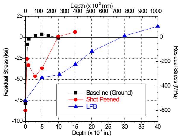
**Figure 16: Residual Stress Distributions for Ground, Shot Peened, and LPB Processed HCF Test Specimens**
