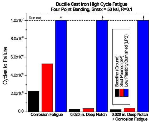
Figure 9: High Cycle Fatigue Results at  $S_{max} = 50$  ksi
