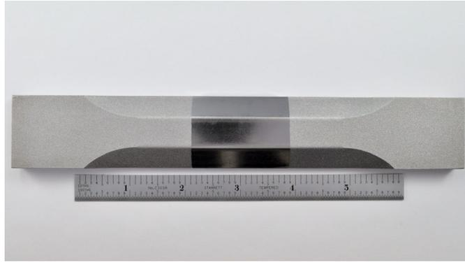
**Figure 1: LPB Processed HCF Specimen**
