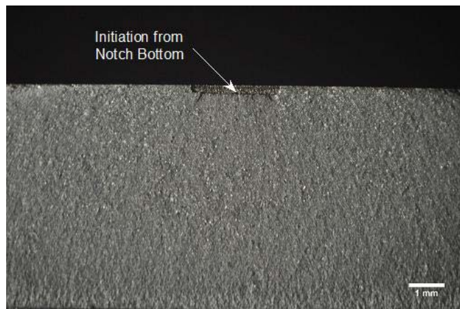
FIGURE 8: FRACTURE FACE OF BASELINE (AS-GROUND) + 0.010 IN. NOTCH SAMPLE.
