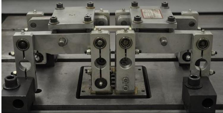
Figure 1: HCF Test Set Up for Testing a Thick Section Specimen.
