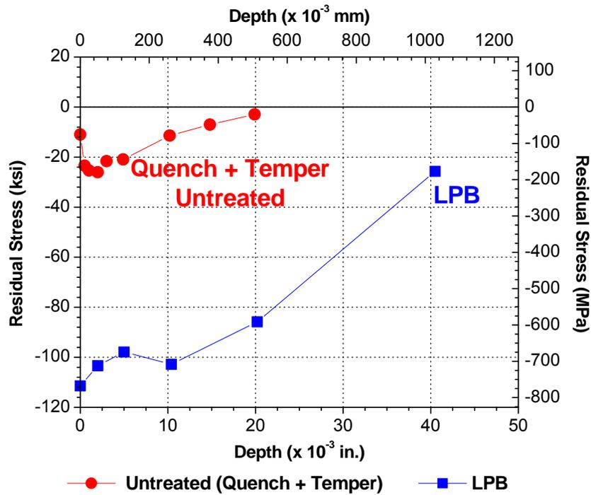
Figure 5: Residual stress comparison for LPB processed and un-treated material.
