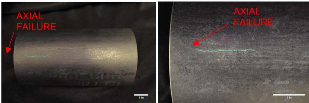
Figure 10: FDI inspection of failed un-treated coupling blank revealing thru wall axial SSC.
