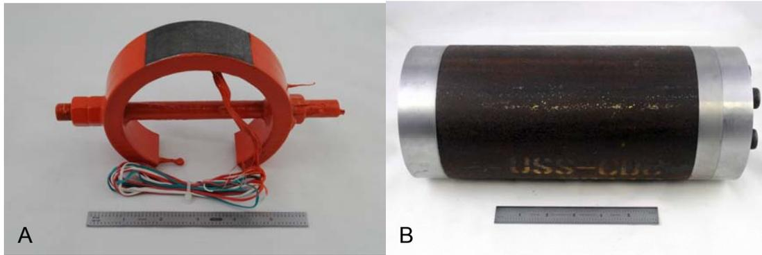
**Figure 2: Examples of tested geometries: (A) C-ring specimen, and (B) full sized coupling blank in test fixture.**
