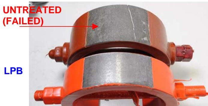
Figure 9: Comparison of LPB treated and un-treated C-ring specimens after testing. The un-treated specimen failed in 10 hours at 45% of SMYS. The LPB specimens ran-out at 45%, 80%, 85%, and 90% SMYS with no cracking.
