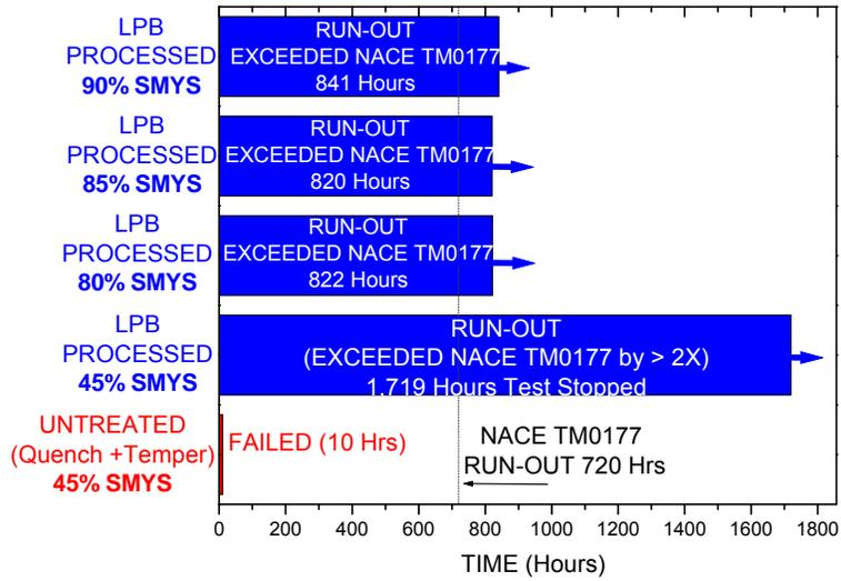
Figure 7: C-ring testing results.
