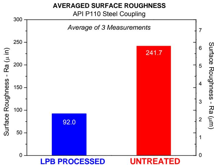
**Figure 6: Surface roughness for LPB processed and un-treated API P110 coupling blank.**
