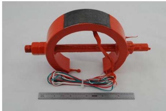
**Figure 3: C-ring specimen prior to testing.**
