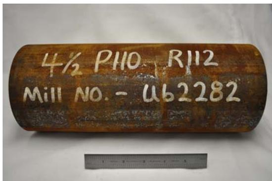
Figure 1: API P110 Quench + Temper coupling stock.
