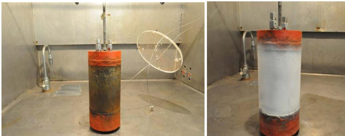
Figure 11: LPB processed coupling blank and test fixture after run-out at 85% SMYS. FDI developer showing no signs of crack initiation.
