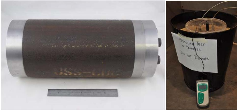
**Figure 4: Full size coupling blank pressurized test apparatus and setup.**
