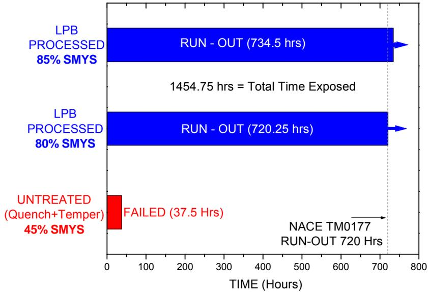
Figure 8: Full Sized Coupling blank Test Results.
