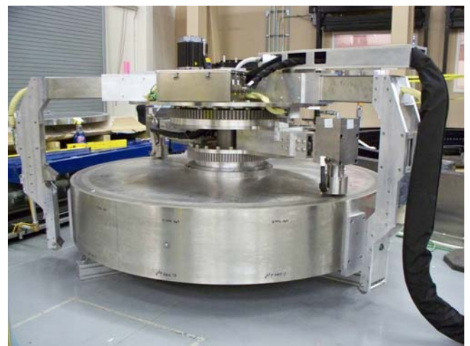
Figure 4: LPB treatment of a nuclear waste containment vessel.
