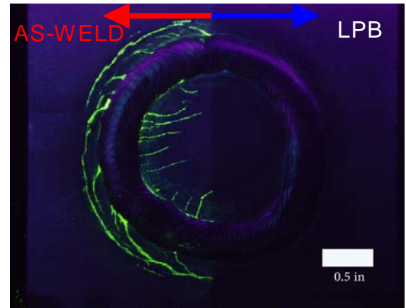
Figure 12. Black light fluorescent dye defines severe SCC cracking on un-treated side of a 316L SS specimen.
