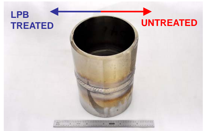
Figure 7.: 316LSS welded pipe specimen; half LPB processed
