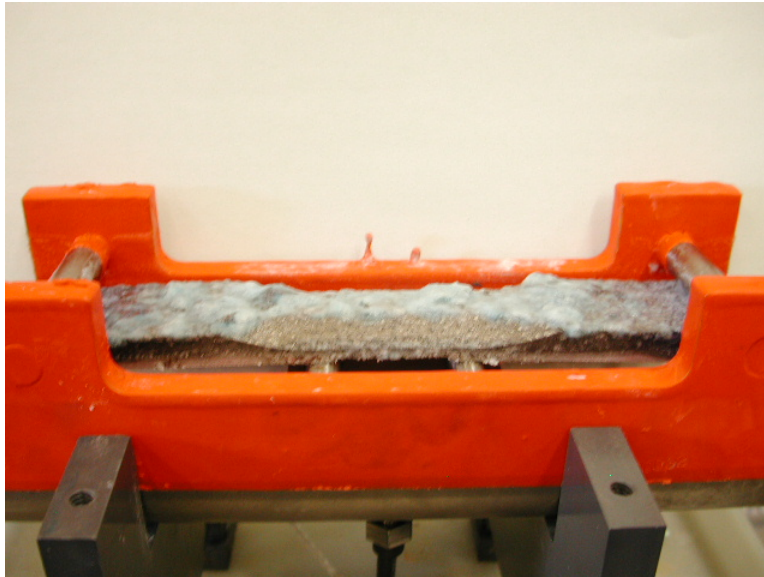
FIGURE 5 - Shot Peened SCC Sample in fixture after testing.
