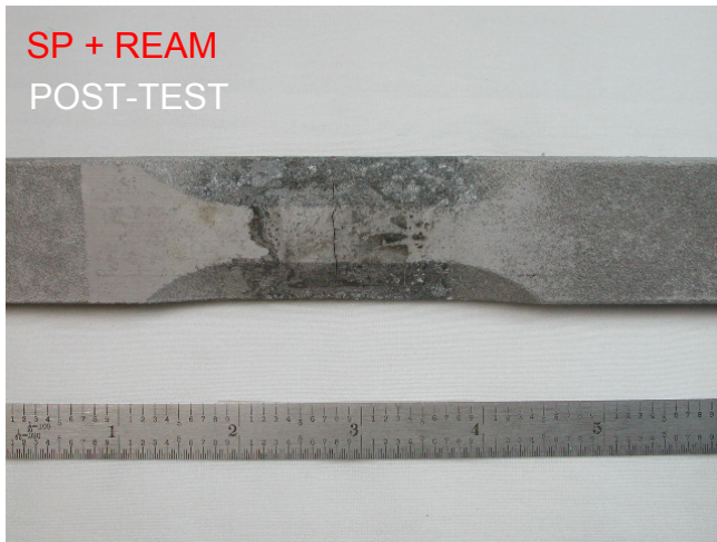
FIGURE 6 – Low magnification photos of specimens before and after exposure. SP specimens exhibited greater damage than LPB specimens.
