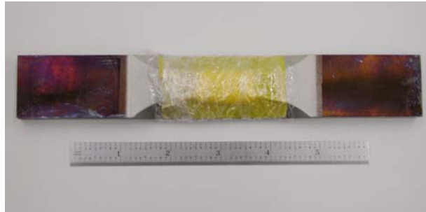
FIGURE 3 - A type 1 HCF specimen with 3.5% salt solution soaked tissue wrapped around the gage section to produce an 'active corrosion' environment during cycling
