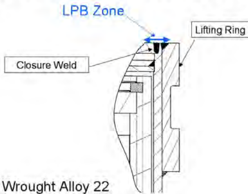
Figure 9.: Alloy 22 closure weld and LPB treatment region
