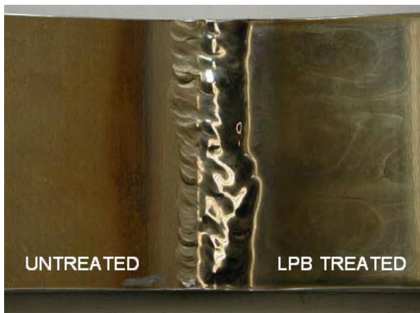
Figure 8.: 304SS welded specimen; half LPB treated
