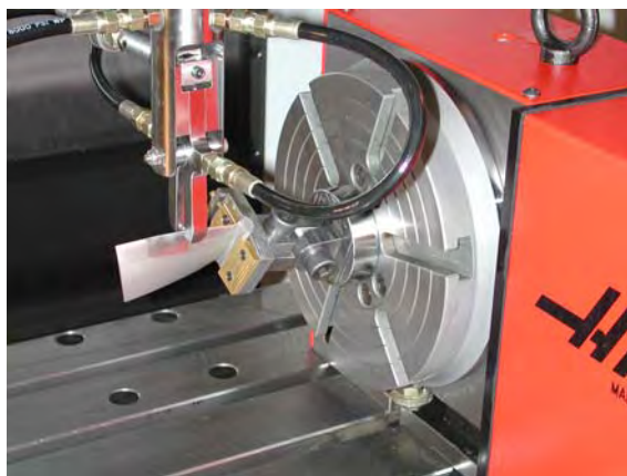
Figure 4. Caliper LPB tool treatment of airfoil leading edge.
