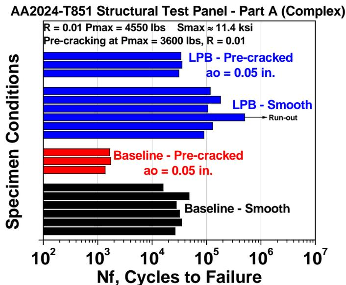
Figure 9. Fatigue life plots for untreated and LPB treated Part A (Complex geometry) tested at  $S_{max} = 11.4$  ksi ( $R = 0.01$ )
