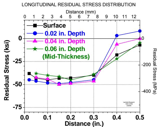
Figure 8. Residual stress distribution in LPB treated Part A.
