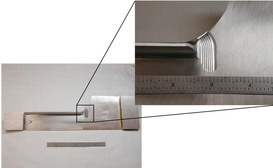
Figure 5. Photographs showing the LPB treated Parts A. Close-up view shows the exact region treated.
