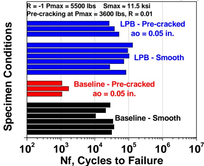
Figure 11. Fatigue life plots for untreated and LPB treated Part B (Simple geometry) tested at  $S_{max} = 11.4 \text{ ksi}$  ( $R = -1$ )
