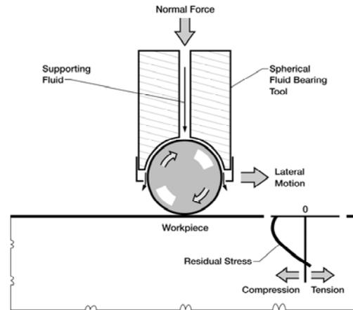
**FIGURE 4 - LPB Schematic**
