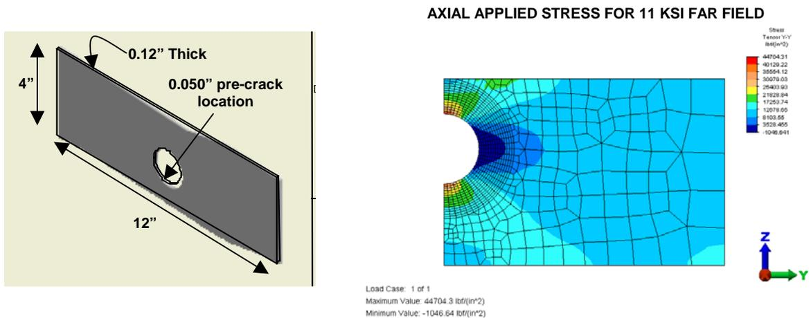
Figure 2. Part B (Simple) geometry and stress contours from finite element analysis (FEA) showing the high stress areas
