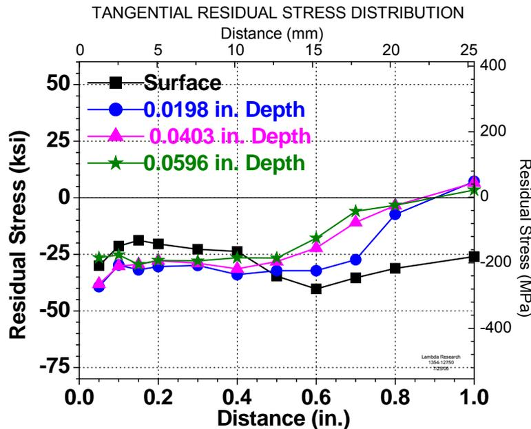
Figure 7. Residual stress distribution in LPB treated Part A.
