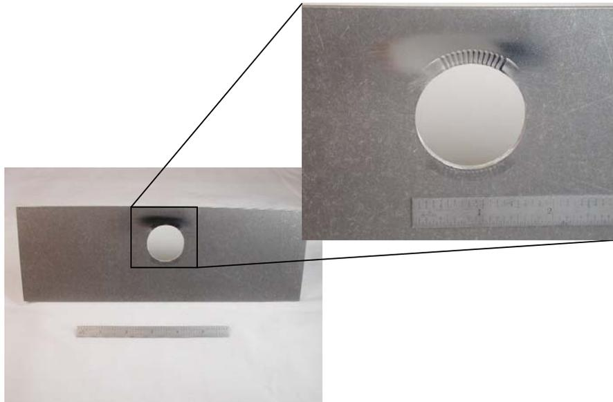
Figure 6. Photographs showing the LPB treated Part B. Close-up view shows the exact regions treated.
