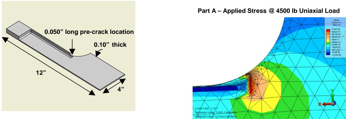
Figure 1. Part A (Complex) geometry and stress contours from finite element analysis (FEA) showing the high stress areas
