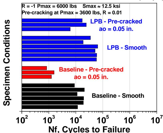
Figure 12. Fatigue life plots for untreated and LPB treated Part B (Simple geometry) tested at  $S_{max} = 12.5$  ksi ( $R = -1$ )
