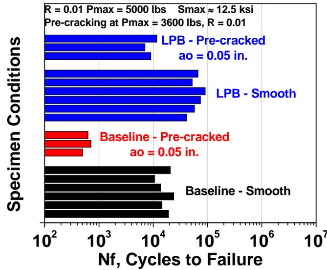
Figure 10. Fatigue life plots for untreated and LPB treated Part A (Complex geometry) tested at  $S_{max} = 12.5 \text{ ksi}$  ( $R = 0.01$ )
