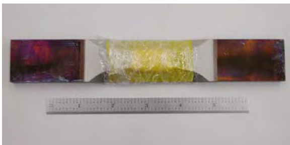
FIGURE 3 - A thick section specimen with 3.5% salt solution soaked tissue wrapped around the gage section.
