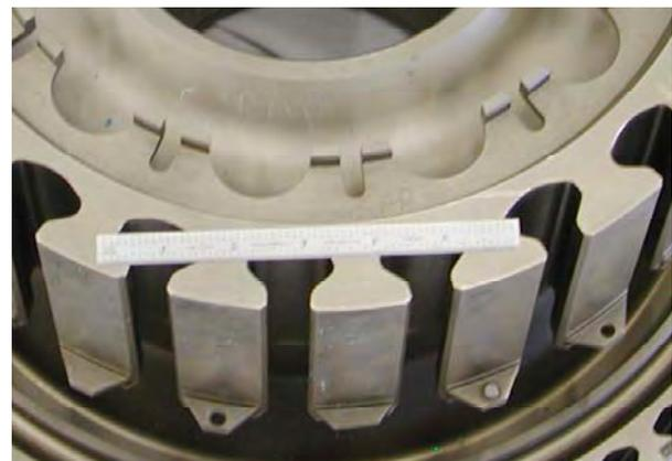
**FIGURE 2** - A close-up view of the dovetail disk post slots.
