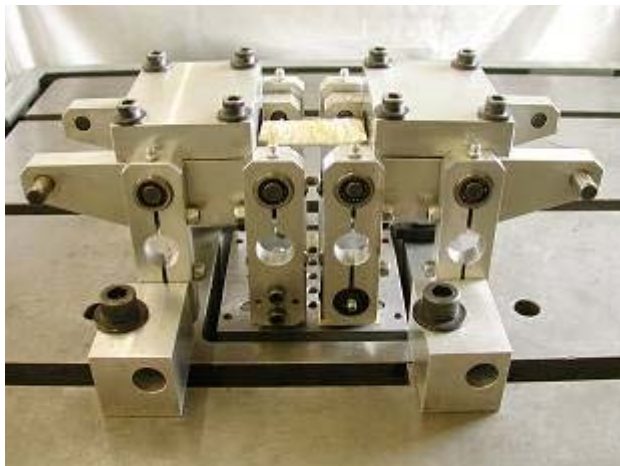
FIGURE 5 - Fatigue test set up.
