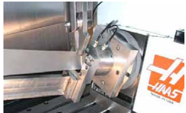
Figure 10. Photograph showing the LPB process set up in a 5-axis CNC milling machine with a caliper tool set ready for LPB processing of the TE of a Ti-6Al-4V compressor vane.
