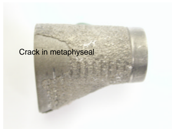
FIG. 7 – Optical photograph of metaphyseal used in conjunction with the testing of sample PR-2003-025-5. Note the cracking in the metaphyseal that occurred before complete failure of the construct.
