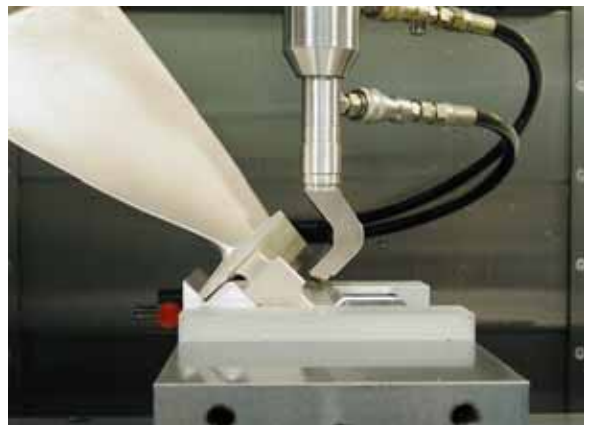
Figure 3 Single point tool LPB processing of the dovetail of Ti-6-4 compressor blade.
