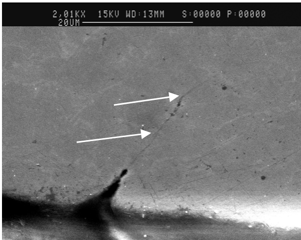
Figure 3. Cross-sectional micrograph of a typical microcrack.
