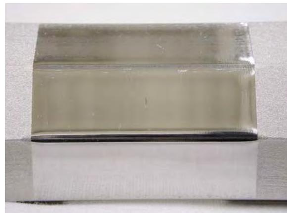
(a) TS Specimen EDM notch,  $a_o = 0.010$  in.,  $c_o = 0.030$  in.
