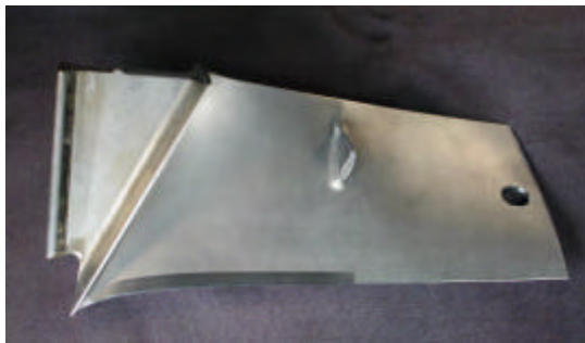
Figure 7 – Photograph of a finished Ti-6Al-4V first stage fan blade showing the LPB region spanning the lower half of the leading edge. (The hole near the tip of the blade is used for loading during fatigue testing.)
