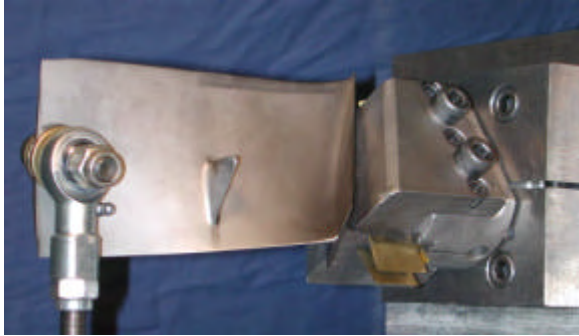
Figure 8 – Close-up of the first stage fan blade mounted in cantilever loading for fatigue testing. (Note the low plasticity burnished leading edge at the top of the blade.)
