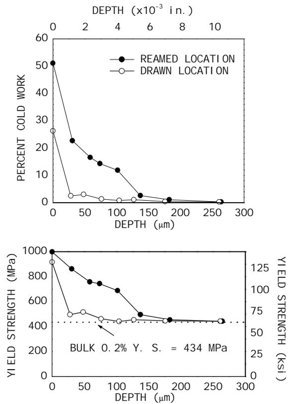
**Fig. 6** Subsurface percent cold work (equivalent accumulated true plastic strain) and corresponding yield strength distribution for baseline drawn and reamed locations on Alloy 600 sleeves removed from service.
