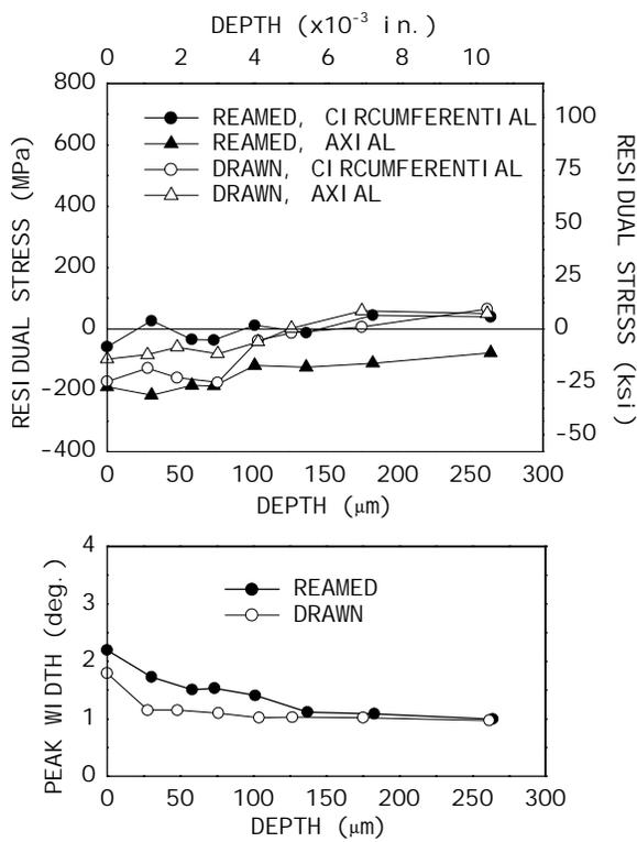
**Fig. 5** - Baseline subsurface axial and circumferential residual stress and (420) peak width distributions for drawn and reamed Inconel 600 sleeve removed from service.
