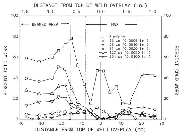
**Fig. 8** Variation in degree of cold work (equivalent accumulated true plastic strain) with axial displacement and depth in the HAZ and machined regions of the low-angle side of the 50° Alloy 600 J-weld mockup
