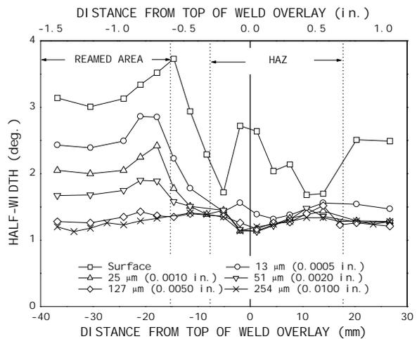
**Fig. 7** Variation in (311) peak width with axial displacement and depth through the HAZ and machined regions on the low side of the 50° Alloy 600 J-weld mockup
