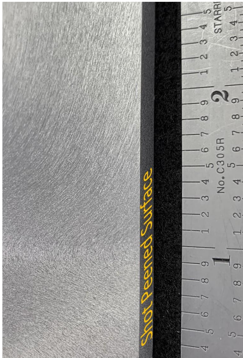
Figure 1: Etched cross section of forged material showing grain orientation and flow near the shot peened surface
