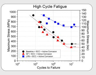
**SOLUTION:** Low Plasticity Burnishing (LPB®) was applied to 410 stainless steel specimens to introduce a deep, stable layer of compressive residual stress in damage-prone regions. X-ray diffraction confirmed surface compression exceeding –100 ksi, with a depth of over 1 mm—far surpassing the reach of common surface damage. Compared to shot peening, LPB-treated samples showed significantly improved high-cycle fatigue strength, with life extended by
