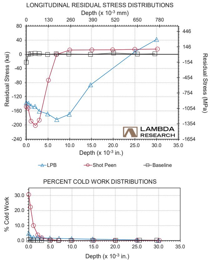
Figure 1: RS vs Depth in Gauge Region
