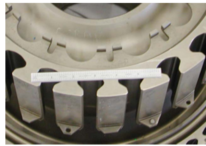
Fig. 2 A close-up view of the dovetail disk post slots
