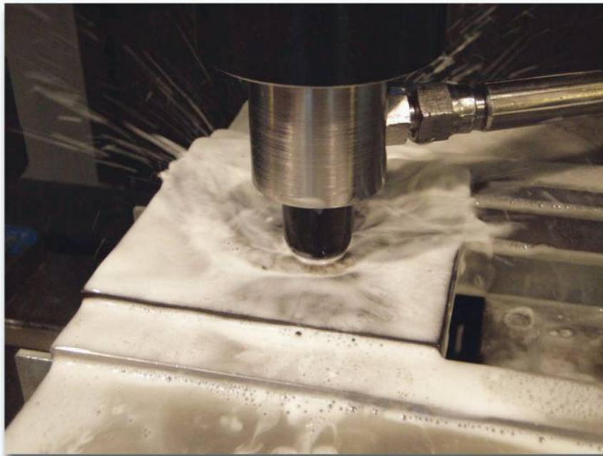
The low plasticity burnishing process uses a hydrostatic tool that continuously “floats” the burnishing ball in fluid during operation, enabling the tool to apply the correct amount of pressure to surfaces with varying topography. Photo courtesy of Lambda Technologies.
