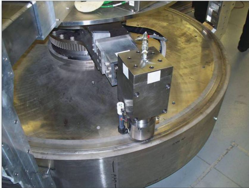
The weld on the top of a nuclear waste container lid, designed for use at a nuclear waste repository, is being treated with low plasticity burnishing to produce residual compression in the fusion weld and heat affected zone. The tool is the device on the top of the lid. Photo courtesy of Lambda Technologies.
