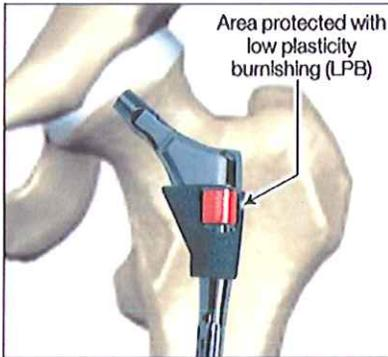
*Fig. 1 — This diagram shows a THP titanium neck segment, metaphyseal (cut away), and femoral stem.*
