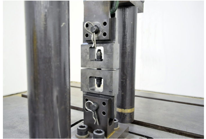
Figure 2: Specimen in Axial Loading on a Sonntag SF-10U HCF Machine
