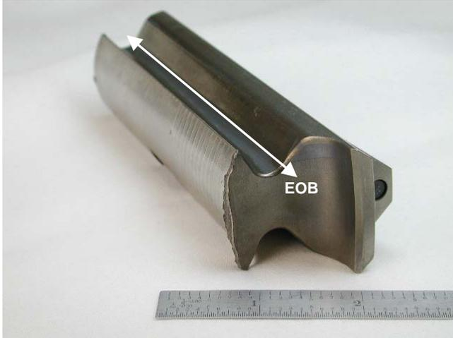
**FIGURE 13** – Photo of the LPB treated disk post. This post was removed from the compressor disk after LPB treatment.
