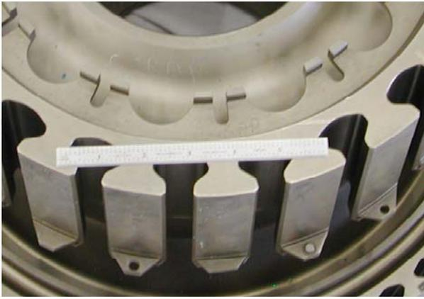
FIGURE 2 - A close-up view of the dovetail disk post slots.
