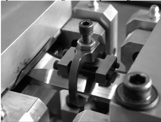
Figure 13 - Photograph of the fretting fixture showing the top two fretting rods clamped onto the top surface of the thick section HCF specimen.
