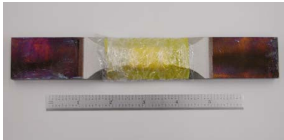
FIGURE 4 - A thick section specimen with salt solution soaked tissue wrapped around the gage section.
